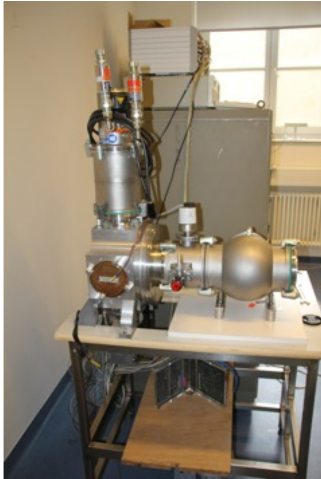
Vacuum chamber and cooling system for one pn-CCD
