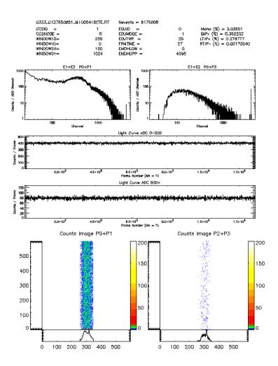
MOS1 U004 bright compressed timing 10:1 Low energy noise, but no missing rows. No counting mode or FTcoarse jump
