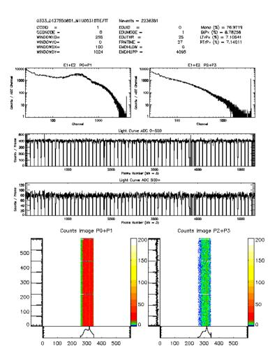
MOS1 U003 bright timing 10:1 event rate 3450/s, bit rate 17.5kb/s Low energy noise and missing rows - not yet understood. Counting mode and FT-coarse jump.
