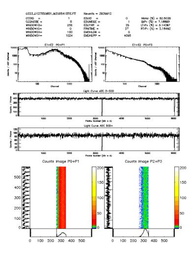
MOS2 U004 bright timing 95:5 Outer CCDs active Event rate 3350/s, bit rate 8kb/s Considerable low energy noise One counting mode glitch No FT-coarse jumps
