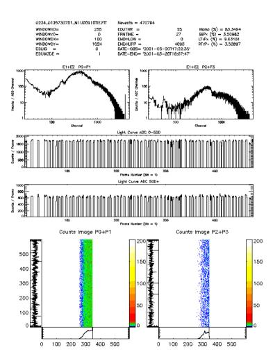
MOS1 U009 Normal timing bin together100 rows Event rate 1300/s, bit rate 64kb/s Some low energy noise. Counting mode and FIFO full errors.
