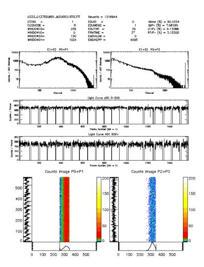
MOS2 U003 bright timing 90:10 Outer CCDs active Event rate 3070/s, bit rate 14kb/s Low energy noise Counting mode and FT-coarse jump.
